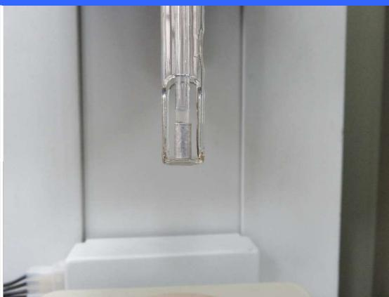
Ruston Services is able to provide high purity aluminium test pieces for thermal analysis expansion work. While this is not a traceable reference material, the high purity of the aluminium pieces ensures that the accuracy of the expansion measurements is high enough for most applications.
