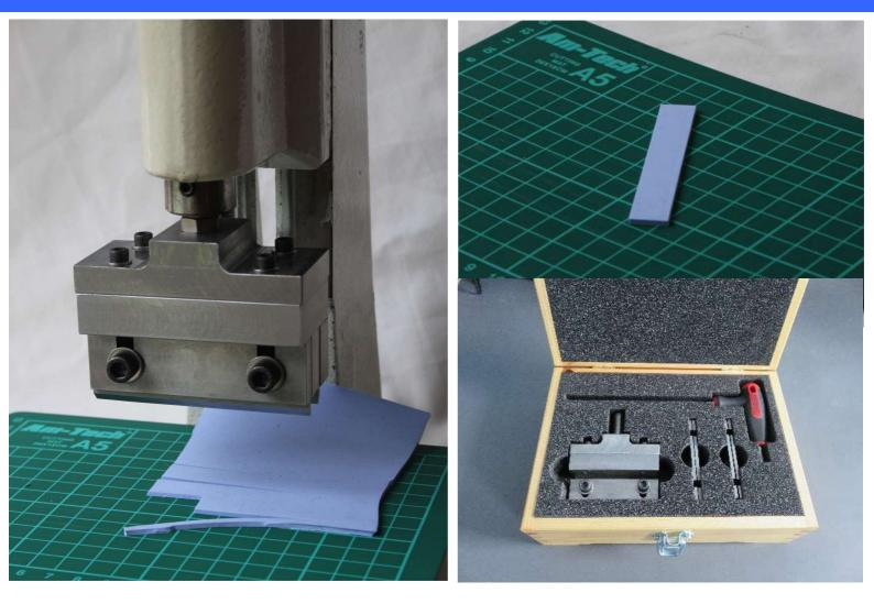
When working with DMA, there is a need to produce parallel samples from the material being studied, and especially in software materials, cutting a suitably accurate sample can be time consuming. To help speed up sample preparation, Ruston Services has developed a parallel cutting tool which has an adjustable sample width setting, allowing a range of materials of different stiffness's to be prepared for analysis by DMA.
