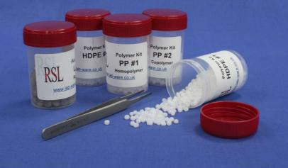
Polymers can be found in all manner of everyday applications, and the materials selected for the polymer kit available from Ruston Services Ltd have been selected to cover a wide range of behaviours. All of the materials have been characterised by experts using FTIR and either DSC or TGA, giving confidence in the data supplied, and separate data sheets are provided for each material when comparing with your own analysis.
