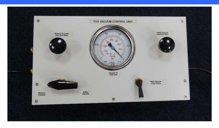
When working under vacuum with Thermogravimetric Analysers (TGA), it is important that the vacuum is both applied and released slowly, otherwise the sample or sample pans can be blown around inside the TGA and cause contamination which requires cleaning out. Ruston Services has designed a suitable manual control panel such that the vacuum can be applied and released using needle valves, with a vacuum gauge which gives a clear indication of the line pressure to the TGA at all times.
