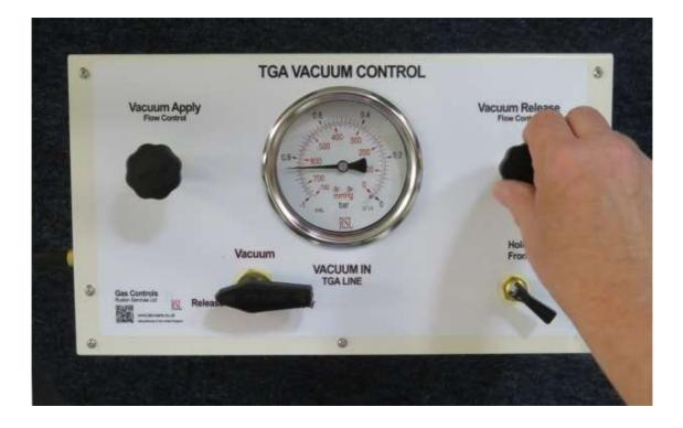
After 1 - 2 minutes, the vacuum in the TGA will be fully released and the gauge will read zero
