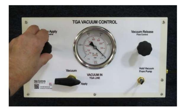
4. When the indicated vacuum falls below 400mm Hg, the Apply Vacuum Gas Flow Rate valve can be slowly opened a little bit more to maintain the speed of evacuation of the TGA.
