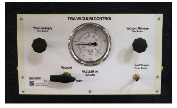
1. Close the Hold Vacuum From Pump valve by lowering the lever to the horizontal position
