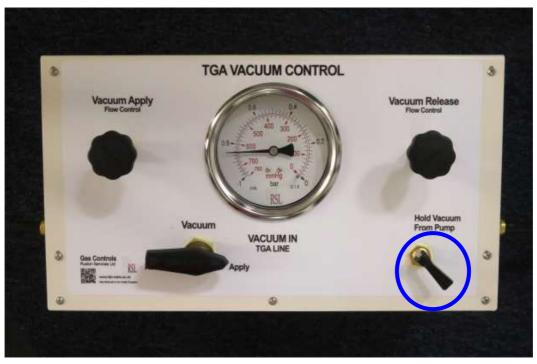
2. Check that the Release Vacuum Gas Flow Rate valve is closed
